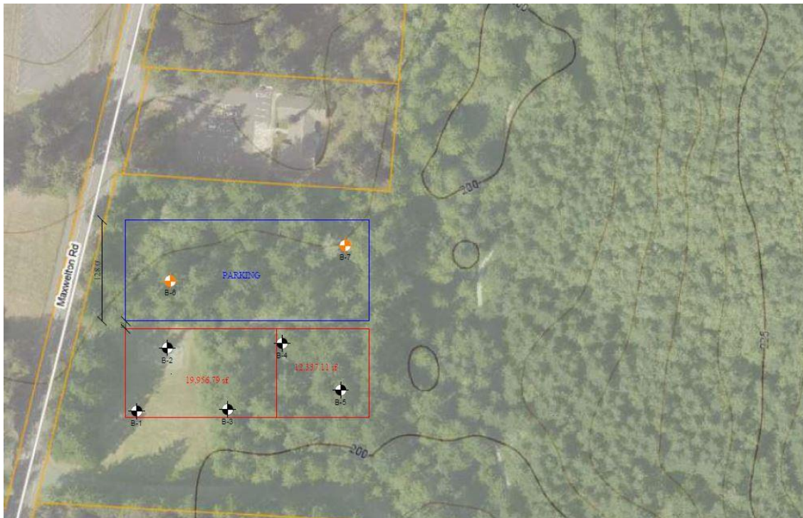
Figure 1: Photo from the Island County Assessor showing an aerial and topographic conditions of project area. Blue area represents parking with two proposed borings and red area represents buildings with five proposed borings.
